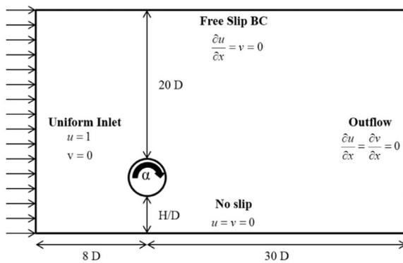
Fig. 1. Schematic diagram of isolated rotating cylinder placed above a plane wall.
