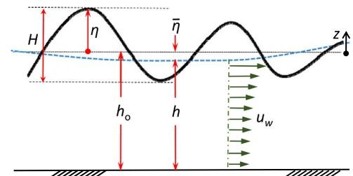
Fig. 1. Definition sketch of wave parameters associated with momentum and mass fluxes through a vertical plane.
