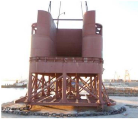
Fig. 1. Rotating wave energy power generation device.
