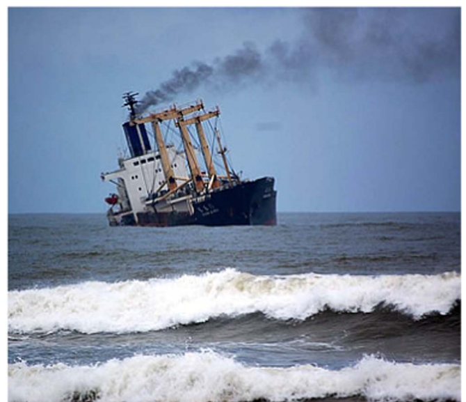
Fig. 3. Bulk Carrier ‘Chang Le Men’ after suspected liquefaction incident off Mangalore India (2007) (Mangalorean, 2007) – see Appendix A.
