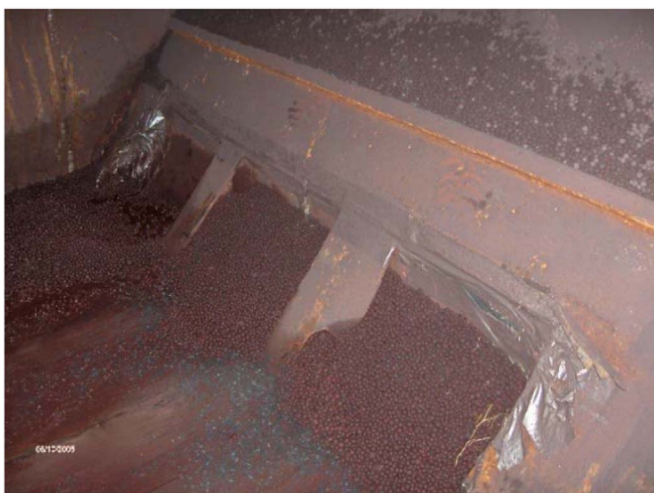
Fig. 2. Three strainer plates blocked by the crew of the Canadian Leader ex Feux Follets using cardboard, plastic sheeting, and duct tape to prevent entry of the cargo of iron ore pellets into the bilge pipes and pumps (Transportation Safety Board of Canada, 2005).
