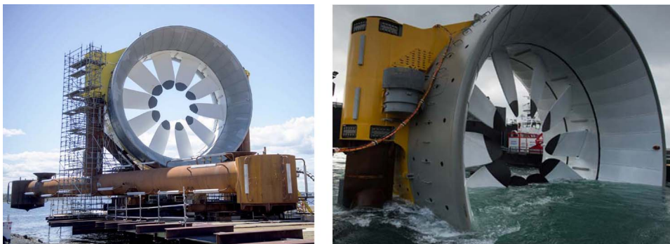
Fig. 1-2. DCNS/OpenHydro 500 kW rated turbine with installation at the Paimpol Bréhat site, Northern France (images credit: DCNS/OpenHydro).
