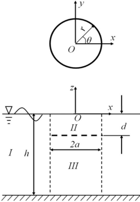
Fig. 1. Definition of the coordinate system and the division of the fluid domain for a submerged horizontal circulate plate.
