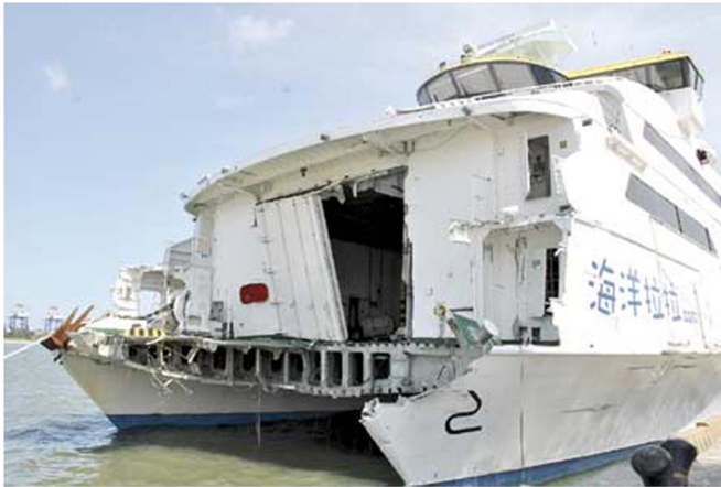
Fig. 1. Damage sustained by Ocean LaLa following an extreme wet-deck slam event on 9th August 2010 en route from Penghu to Taichung. 311 passengers and 22 crew were on-board the vessel when Mayday was sent at 19:04 local time 8.7 miles from port. Although there were no serious injuries recorded, 8 passengers were sent to hospital. ( http://www.chinapost.com.tw/taiwan/national/national-news/2010/08/10/268041/Ferry-accident.htm ).
