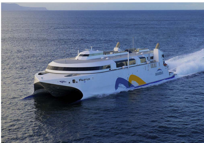
Fig. 2. INCAT Hull 069 – Liquefied Natural Gas (LNG) 99 m wave-piercer catamaran commissioned in June 2013.
