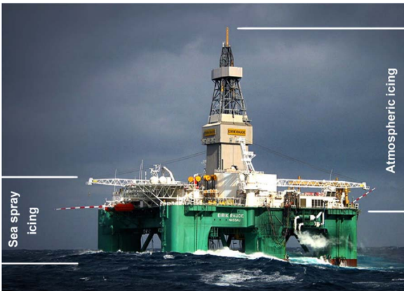
Fig. 3. Ice accumulation regions, through ice type, on the Ocean Rig semi-submersible Eirik Raude (Paulin, 2008; Ryerson, 2011).
