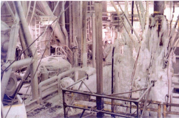
Fig. 2. Sea spray icing on the Ocean Bounty in the winter of 1979–1980 in Lower Cook Inlet (Jones and Andreas, 2009).
