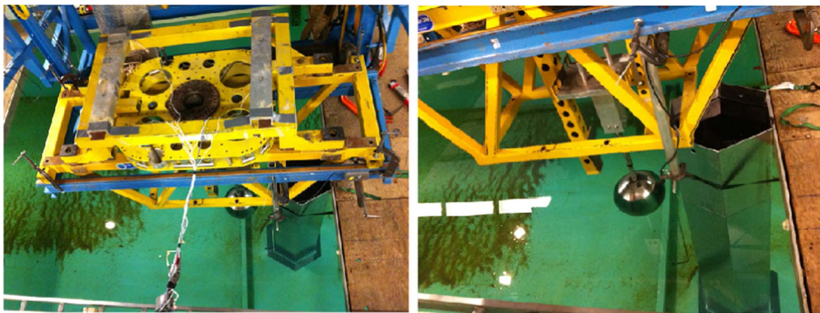
Fig. 2. Experimental set up – dynamometer, fixed structure and sphere D_i/D_s=0.6 .
