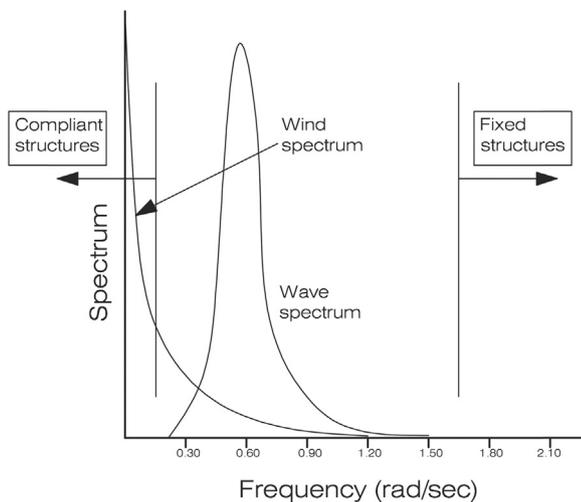
Fig. 1. Excitation and frequency ranges of offshore platforms.
