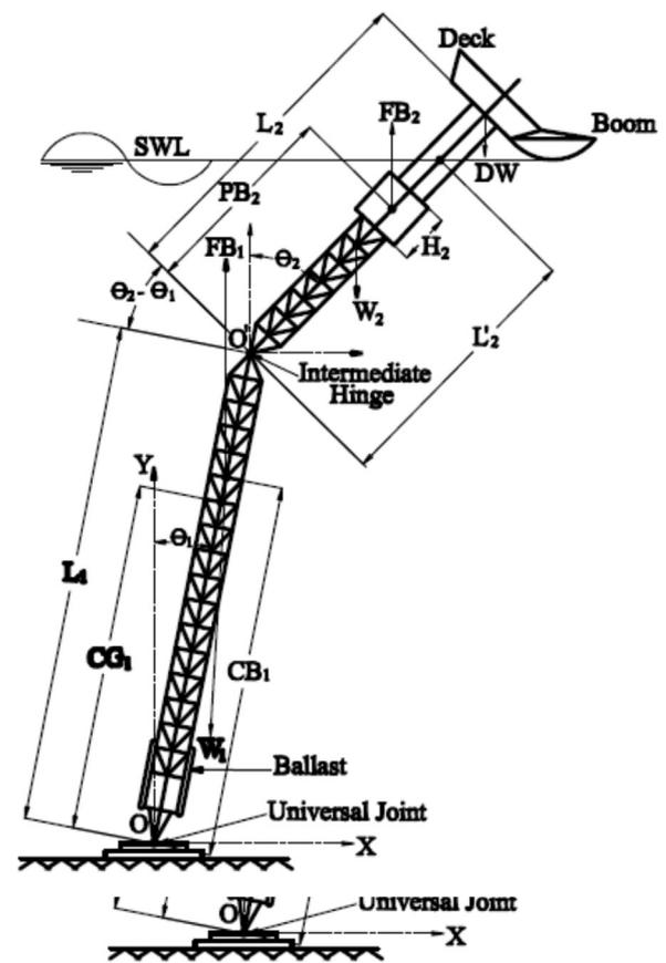
Fig. 2. Mathematical model of double hinged articulated tower.
