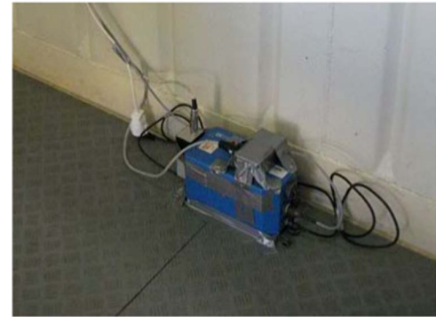
Fig. 2. Fiber optic gyro with rate gyro and heave accelerometer.
