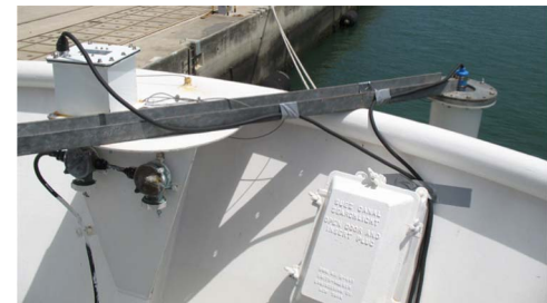
Fig. 3. Bow mounted down-looking wave radar with vertical accelerometer for motion compensation.
