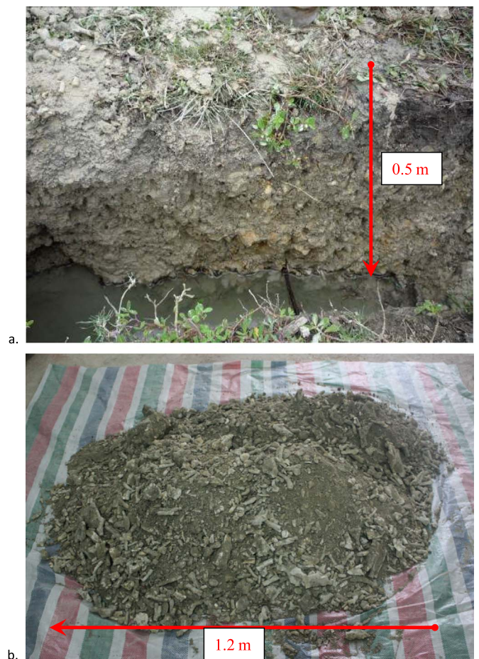
Fig. 3. (a) Geological profile of test GROUPS 2# and 3#; (b) Lagoon soil (clayed sand with gravel, mixed with terrestrial deposits).
