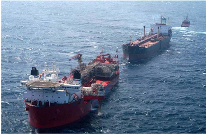
Fig. 1. Tandem offloading operation between a FPSO and a shuttle tanker ( www.zebecmarine.com ).
