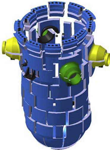
Fig. 1. Example segmentation plan of RPV.
