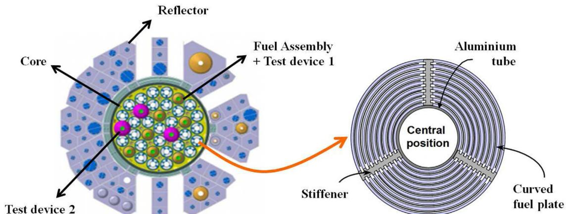
Fig. 1. Schematic of the JHR core and fuel assembly. Courtesy of CEA.
