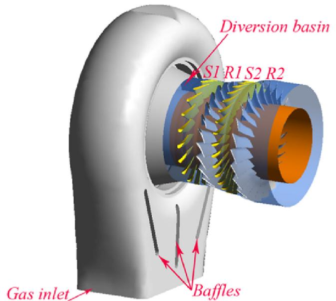
Fig. 1. Intake volute and cascade channel structure of TRT.
