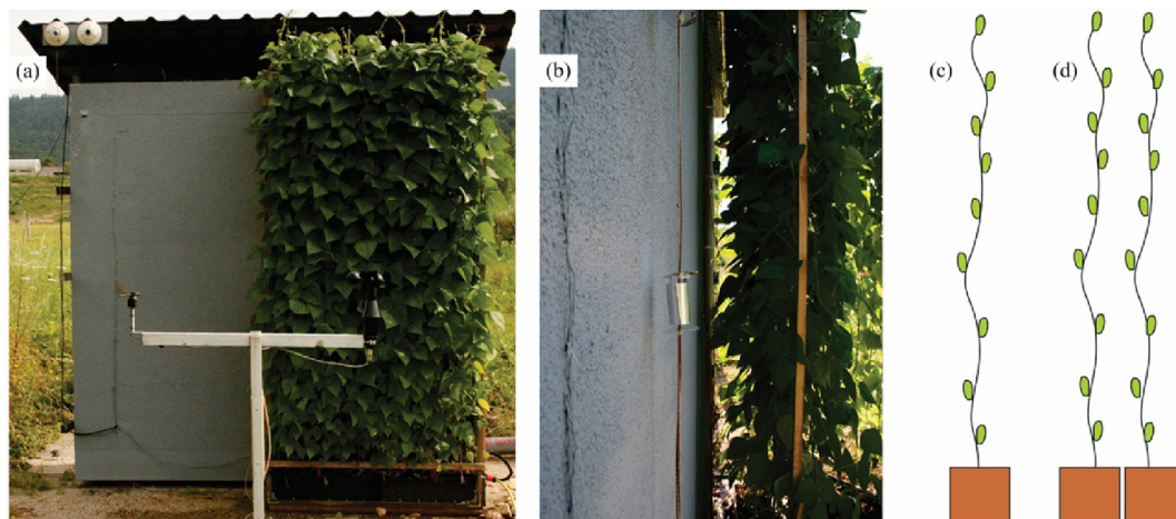
Fig. 1. A front view of the experiment with the thermo-stated test cell with and without the VGS (a), a side-view of the VGS positioned at the thermo-stated test cell (b), a schematic of the one-layered (c) and the two-layered VGS (d).
