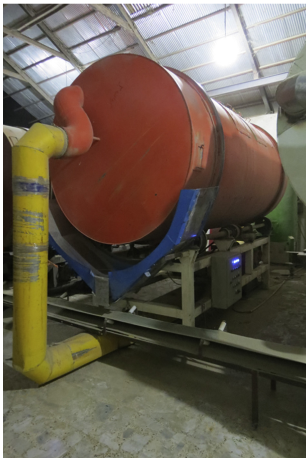
Fig. 1. Industrial horizontal rotary paddy dryer (IHRD).
