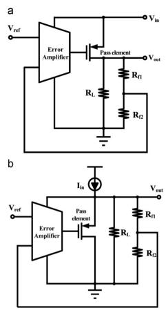
Fig. 1. (a) Series topologies and (b) shunt topologies.
