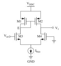
Fig. 3. The trans-conductor circuit Gm-stage of the proposed shunt regulator.
