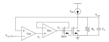
Fig. 2. Block diagram of the proposed shunt regulator.
