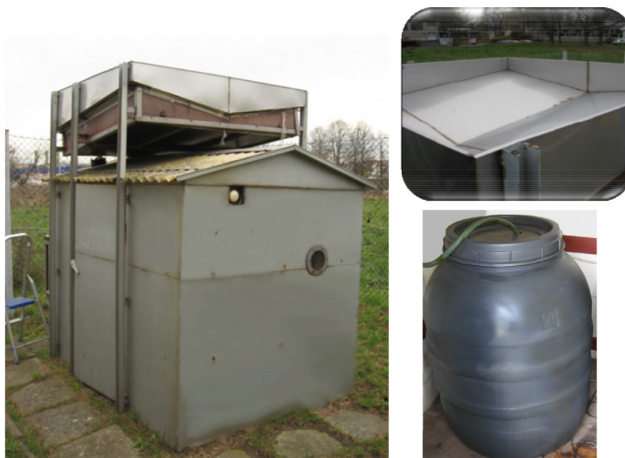
Fig. 1. Photo of air precipitation collector designed at IFJ PAN in Krakow and used to collect samples for present paper (left). Right top – the view on stainless steel trap, Right bottom – 160 L plastic barrel used for storing the sample. .
