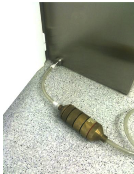
Fig. 3. Test of the decontamination capacity of the activated carbon filter combination in the filter unit to the right of the fume hood via a removal device (tubing joint) was fitted.
