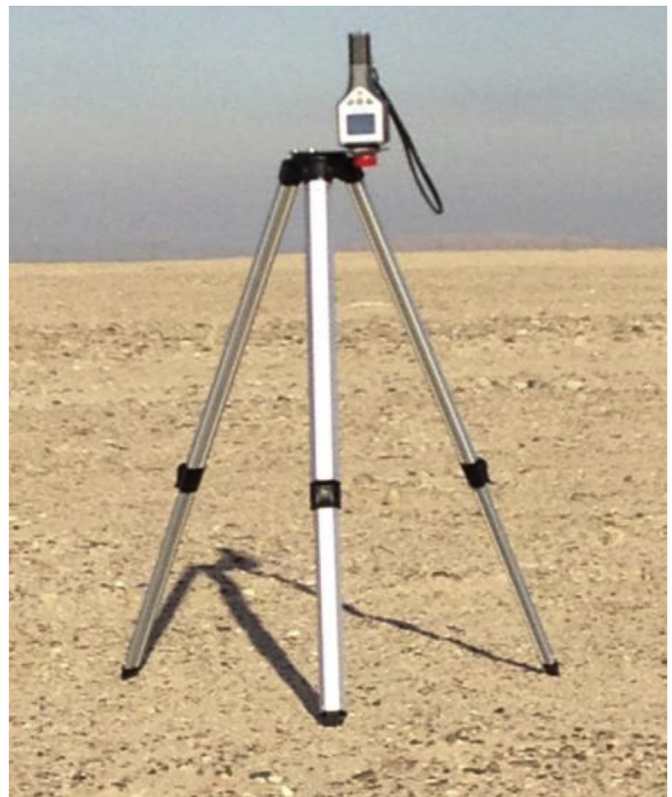
Fig. 1. The handheld NaI dosimeter/spectrometer “ identiFINDER 2 ” on a tripod at the height of 1-meter in one of the northern locations in the desert of Kuwait.
