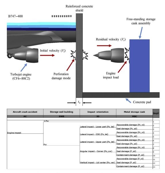
Fig. 1 – Illustration of impact scenario with aircraft crash event tree model.
