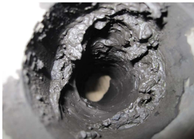
Fig. 2. Precipitated solids, derived from algal biomass ( Tetraselmis sp.), collected in the HTL reactor filter trap.
