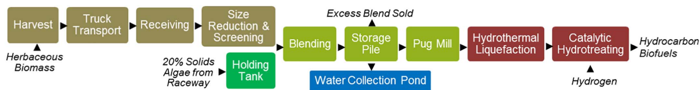
Fig. 1. Flow diagram of unit operations. Herbaceous biomass, harvested from the field and delivered by truck to a receiving area, undergoes preprocessing operations to meet size and ash specifications. Harvested algae (20% solids, db) in excess of conversion capacity is transferred to a holding tank, then mixed with herbaceous biomass and added to a storage pile. Upon retrieval from storage, the blend is reconstituted to 20% solids (db) so that it can be fed into the HTL reactor, followed by catalytic hydrotreating to form hydrocarbon biofuels. Excess blend remaining in the storage pile is sold once capacity in the HTL reactor has been maximized.
