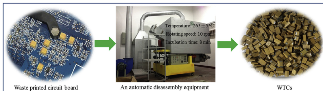
Fig. 3. An automatic system for WTCs disassembly from WPCBs.
