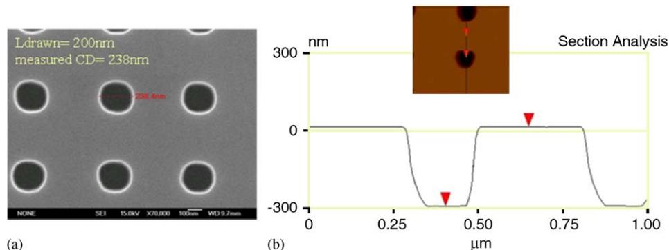
Fig. 1. (a) 2D array of via holes with 238 nm of measured CD and (b) AFM image with a line scan result showing a flat bottom profile and slightly higher vertical distance (~308 nm) than deposited SiO<sub>2</sub> thickness.
