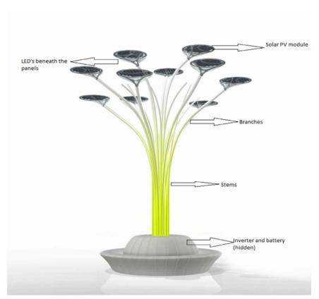
Fig. 1. Common layout of a solar tree [24].
