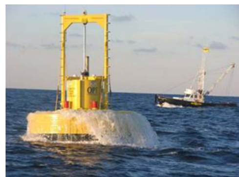
Fig. 4. OPT PowerBuoy wave energy generation system (US). Adapted from [12].
