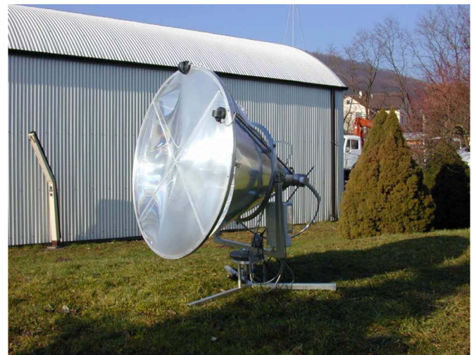
Fig. 2. A SOLUX collector without the protecting acrylic dome [15].
