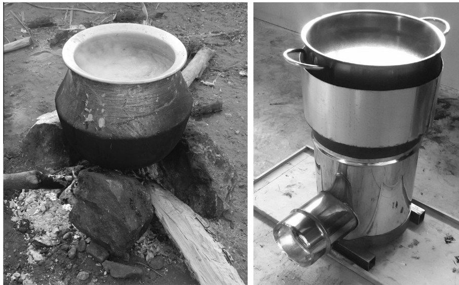
Fig. 1. Examples of TSF (a) and ICS (Rocket model) (b).
