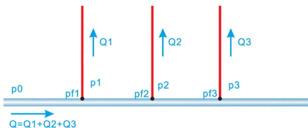
Fig. 1. Schematic representation of fluid distribution for multiple perforation clusters in a horizontal well (a half of the model).
