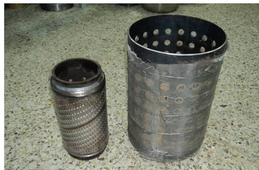
Fig. 2. Gravel packing combination for 52 mm gravel thickness (tests 3, 4 and 8).
