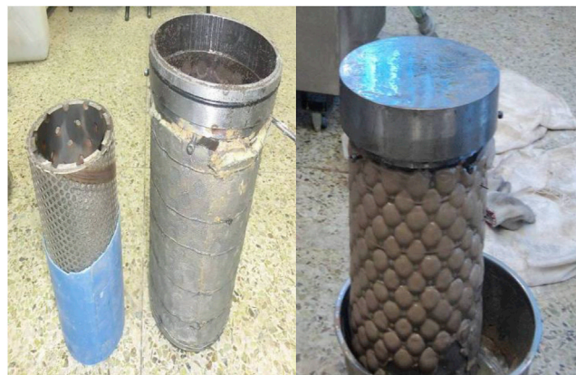
Fig. 3. Gravel packing combination for 38 mm gravel thickness (tests 2, 6 and 7).
