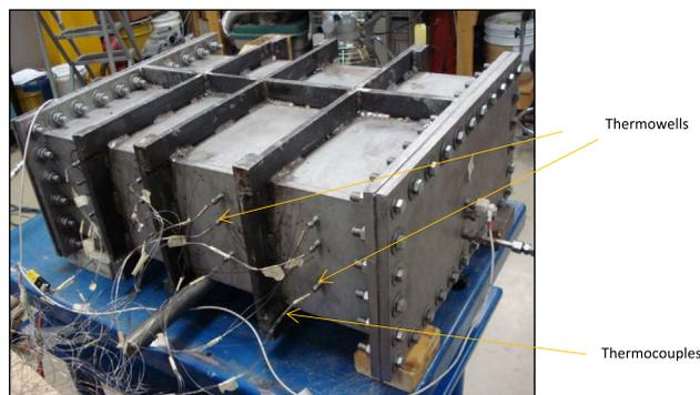
Fig. 1. Photograph of CAGD cell. The ends of the cell may be removed to introduce sand mix or to clean out burnt sand after an experiment. A total of 48 thermocouples are placed inside the thermowell that are installed on two sides of the cell.
