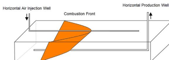
Fig. 2. The combustion front is initiated near the heel of the injection well and follows the path of the injector. Mobilized oil is drained to the lower horizontal producer by gravity drainage.
