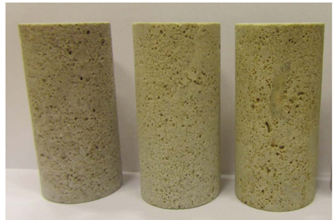
Fig. 1. Silurian dolomite samples of 1.5 in. diameter and 3 in. length.
