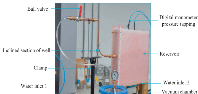
Fig. 1. Water and gas cresting facility.
