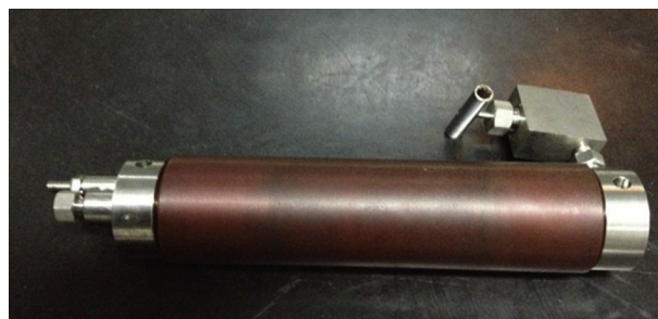
Fig. 1. Core holder made of carbon fiber.
