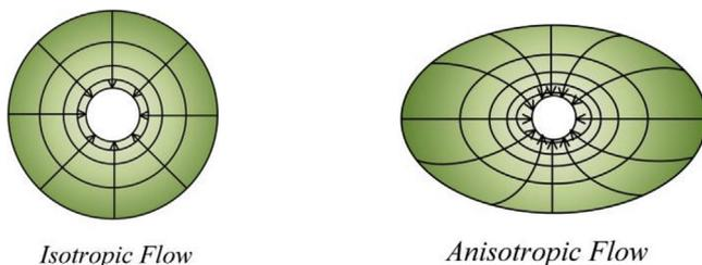
Fig. 1. Sketches of isotropic and anisotropic flow.
