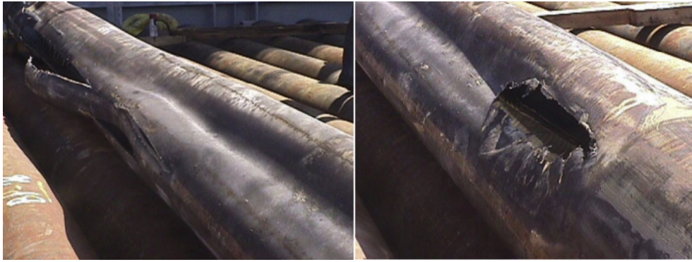
Fig. 1. The collapsed casings in deepwater oil and gas well (Bradford et al., 2002; Bradford et al., 2004).
