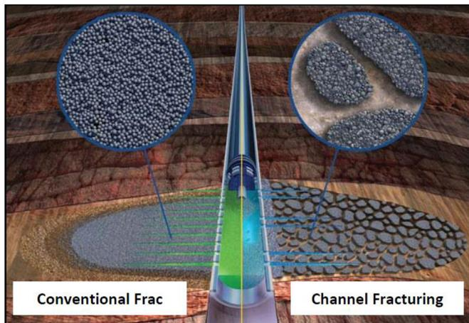
Fig. 1. Comparison of channel fracturing and conventional fracturing (Gillard et al. 2010).
