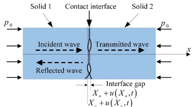
Fig. 1. Schematic model of longitudinal wave propagating through a contact interface between two linear elastic solids [52,54].
