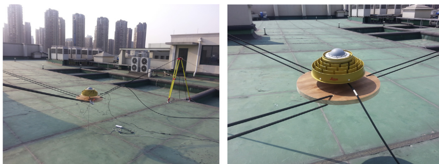
Fig. 1. The bungee experiment located on the roof of the Science and Engineering Building, UNNC (left), and a close up view of the Leica AR25 choke ring GNSS antenna (right).
