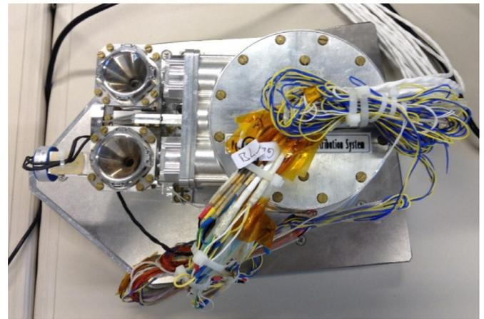
Fig. 1. PSDDS breadboard model as configured for the sample cementation tests.
