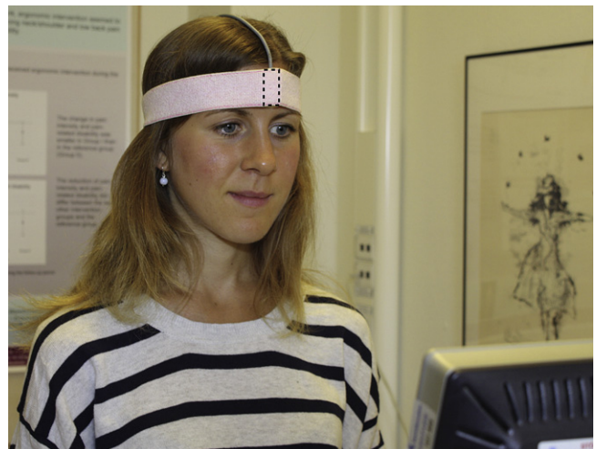
Fig. 1. A triaxial accelerometer sensor was taped to the skin on the forehead and secured with a headband.
