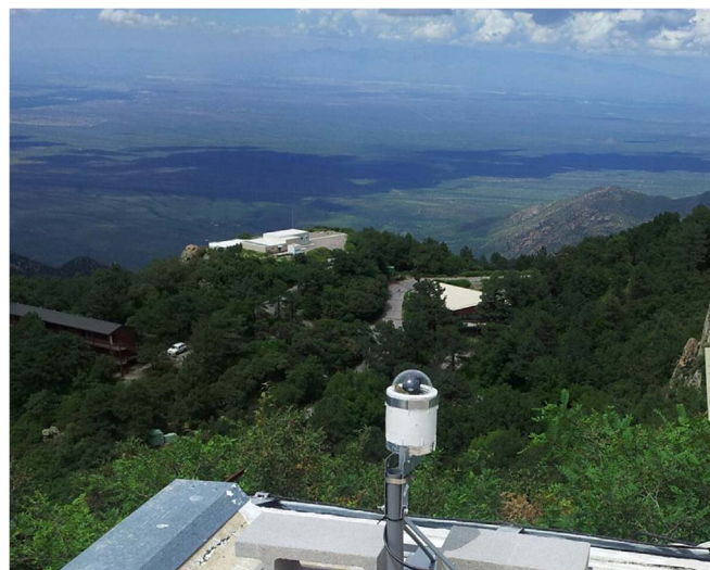
Fig. 2. NASA All Sky Fireball Network meteor camera, pictured here on the roof of a building near Tucson, Arizona.
