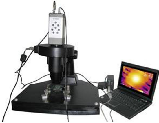
Fig. 1. Optical micro-scanning thermal microscope imaging system.
