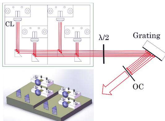
Fig. 1. The scheme of EC beam combining of QCLs. Both 2D and 3D sketch maps are showed.
