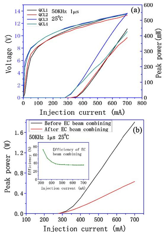
Fig. 2. (a) Four different QCLs peak power versus the injection current of in pulse mode at a condition of 5% duty circle and 1  $\mu\text{s}$  pulse width along with the V-I curves at 25  $^\circ\text{C}$ . (b) Optical peak power as a function of current for the total power and the beam-combined output power. The inset shows the beam combining efficiency changes with the injection current.
