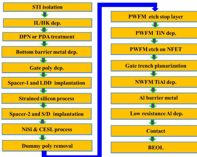
Fig. 2. Simple process flow of 28 nm gate-last MOSFET devices.
