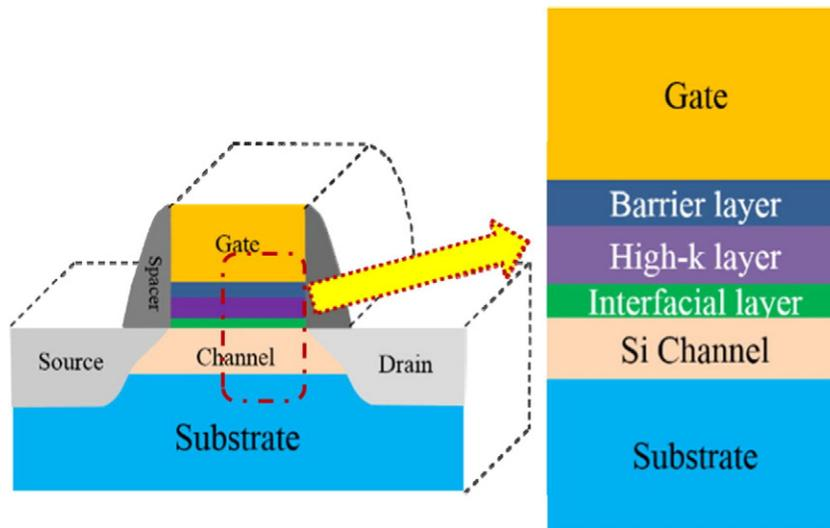
Fig. 1. Schematic cross-section profile of an nMOSFET.
