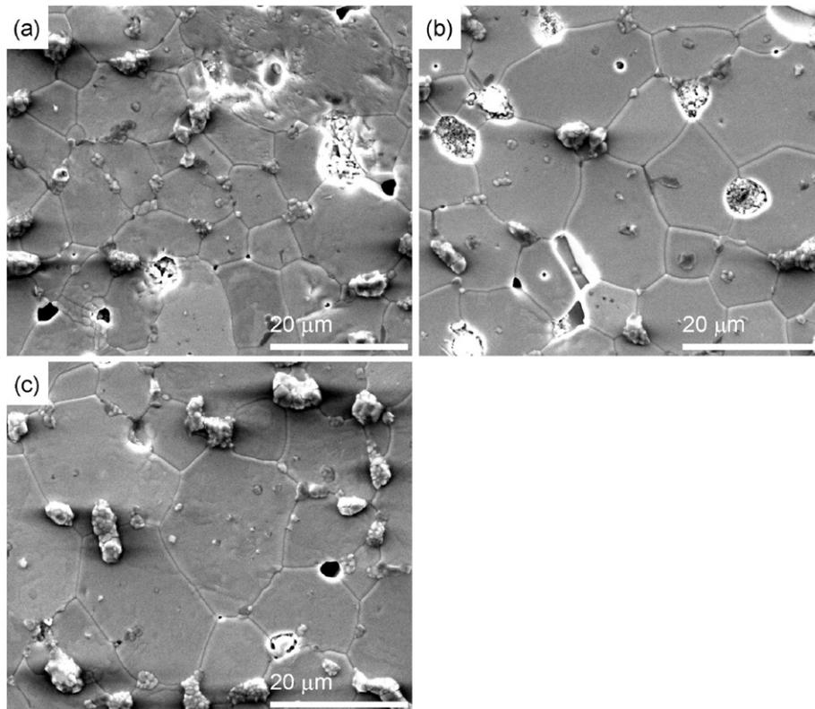
Fig. 1. SEM micrographs of the samples with different sintering times; (a) 1 h, (b) 2 h, and (c) 3 h.
