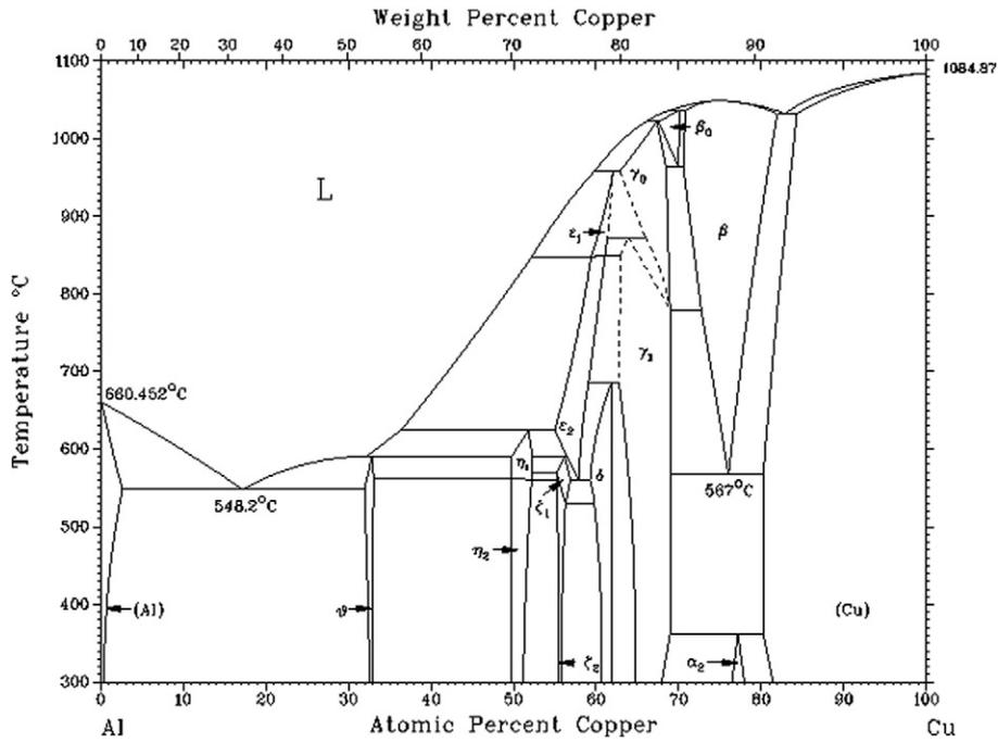
Fig. 1. Cu–Al phase diagram.
