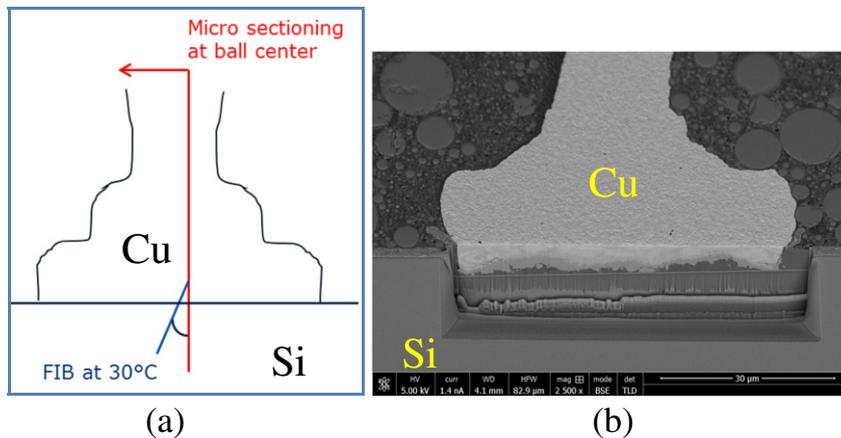
Fig. 2. Sample preparation for group A. (a) Schematic diagram of the microsectioning direction at ball center followed by FIB cut at 30 °C. (b) FIB overview at the entire ball interface after FIB cut.
